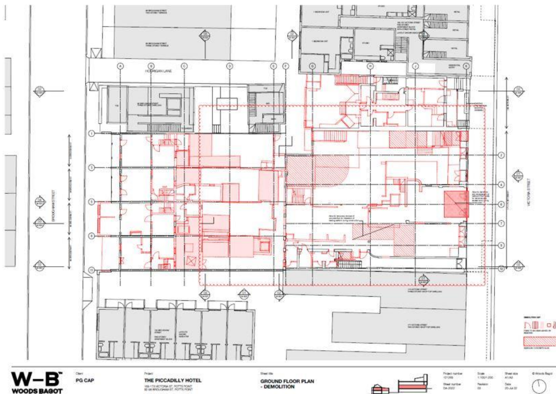
Figure 24: Proposed ground floor demolition floor plan drawing extract
