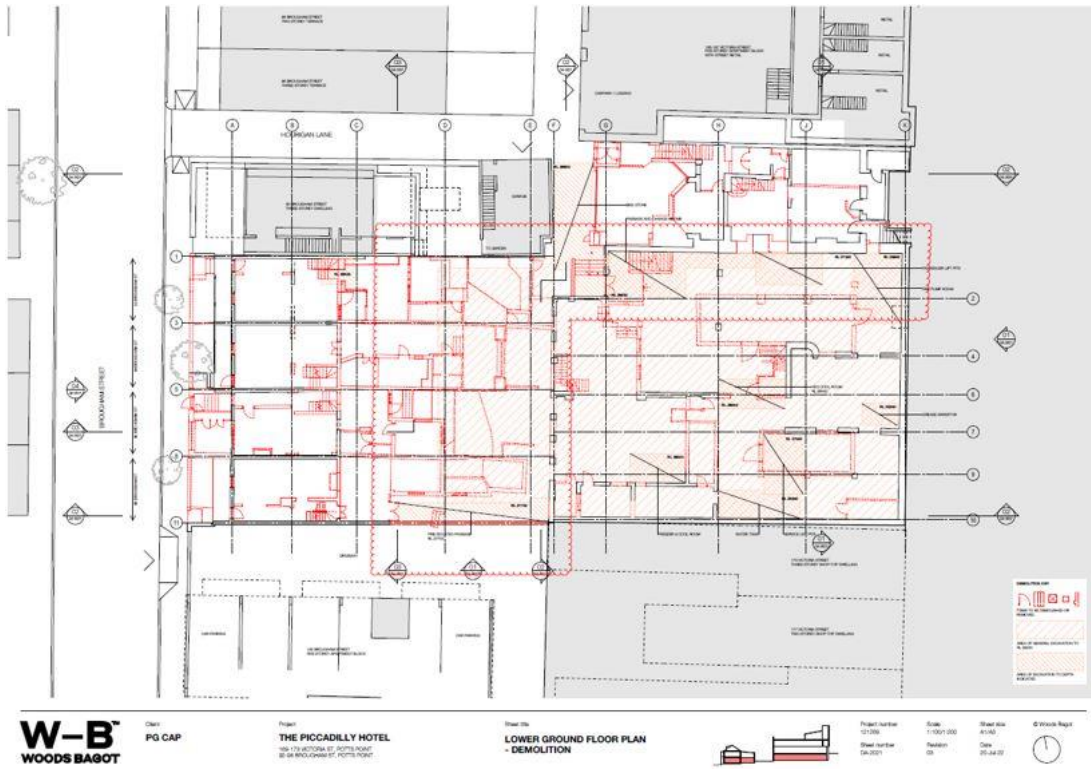
Figure 23: Proposed lower ground floor demolition floor plan drawing extract
